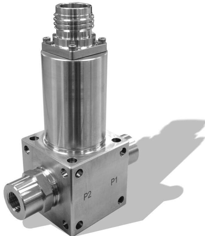
The 226-30-0020 Series CANopen<sup>®</sup> Submersible Differential Transmitters offer precise pressure measurement of liquids and gases from 0-10,000 PSID (690 BAR), with the added value of temperature measurements from +25 °F to +175 °F (-4 °C to +80 °C).
