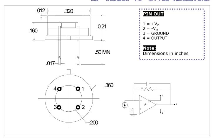
The preamplifier portion of this receiver is a transimpedence current to voltage converter. Its output voltage is proportional to the input signal current:
