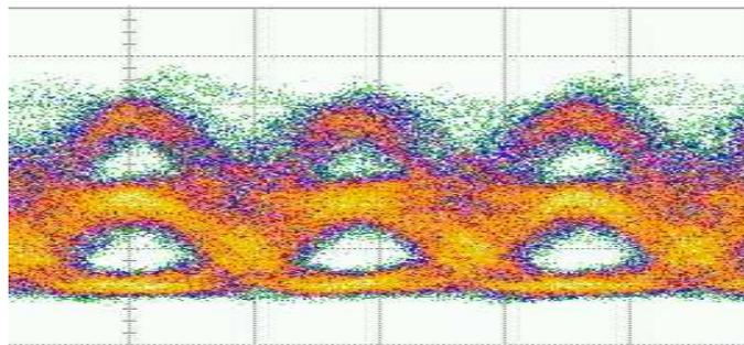
Figure 2: Eye diagram of the QAM16 signal emulated
